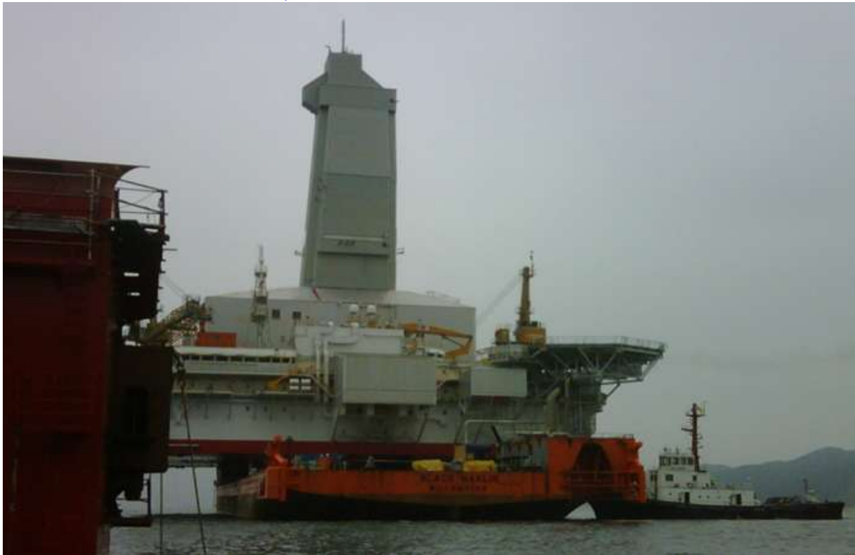
Dockwises' Black Marlin carrying the 19.000mT Gazflot " Polyarnaya Zvezda " topside seen from the Hull about to start first float over operation for Vyborg. Photo : John van der Woning (c)
