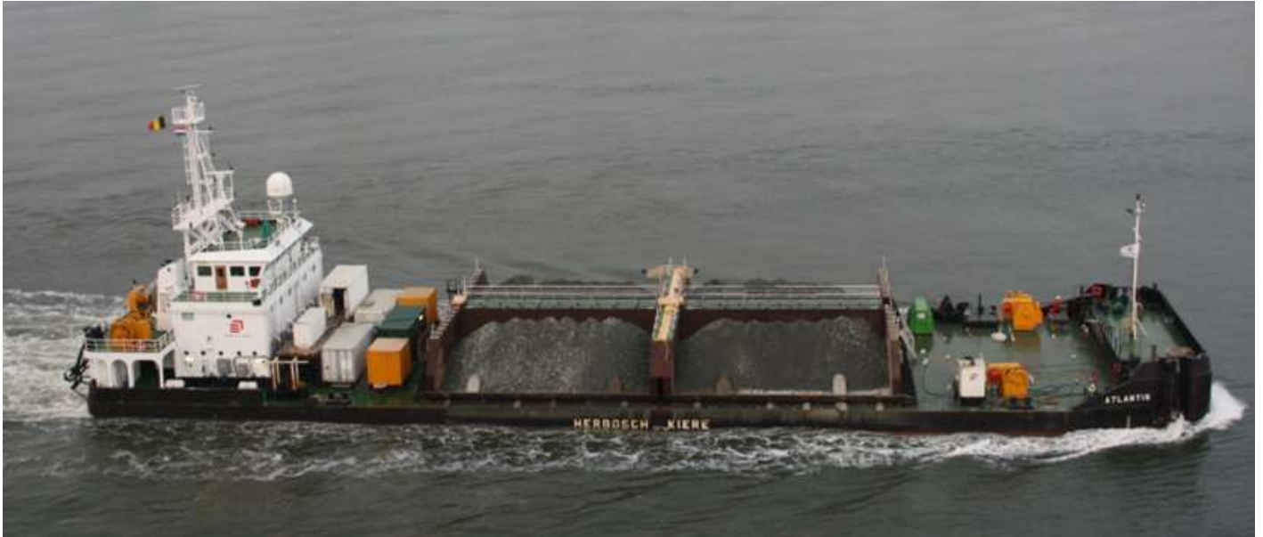
The Belgian flagged ATLANTIS is used for rock / stone dumping at the Maasvlakte II project Photo : Rik van Marle ©
